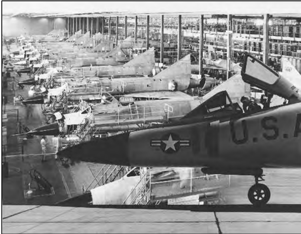
Figure 4.2-12 F-102 Assembly Line Courtesy of San Diego Air and Space Museum.
