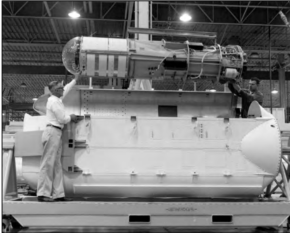
Figure 4.2-49 Placing OV-1 in Satellite in Dual Ejection Pod Courtesy of San Diego Air and Space Museum.
