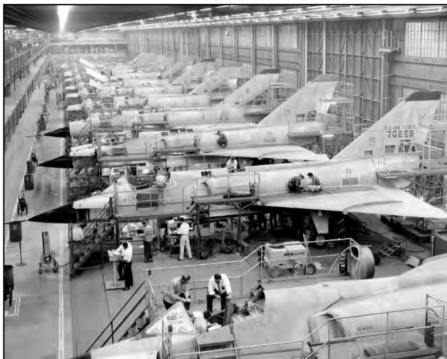
Figure 4.2-15 F-106 Assembly Line Courtesy of San Diego Air and Space Museum.
