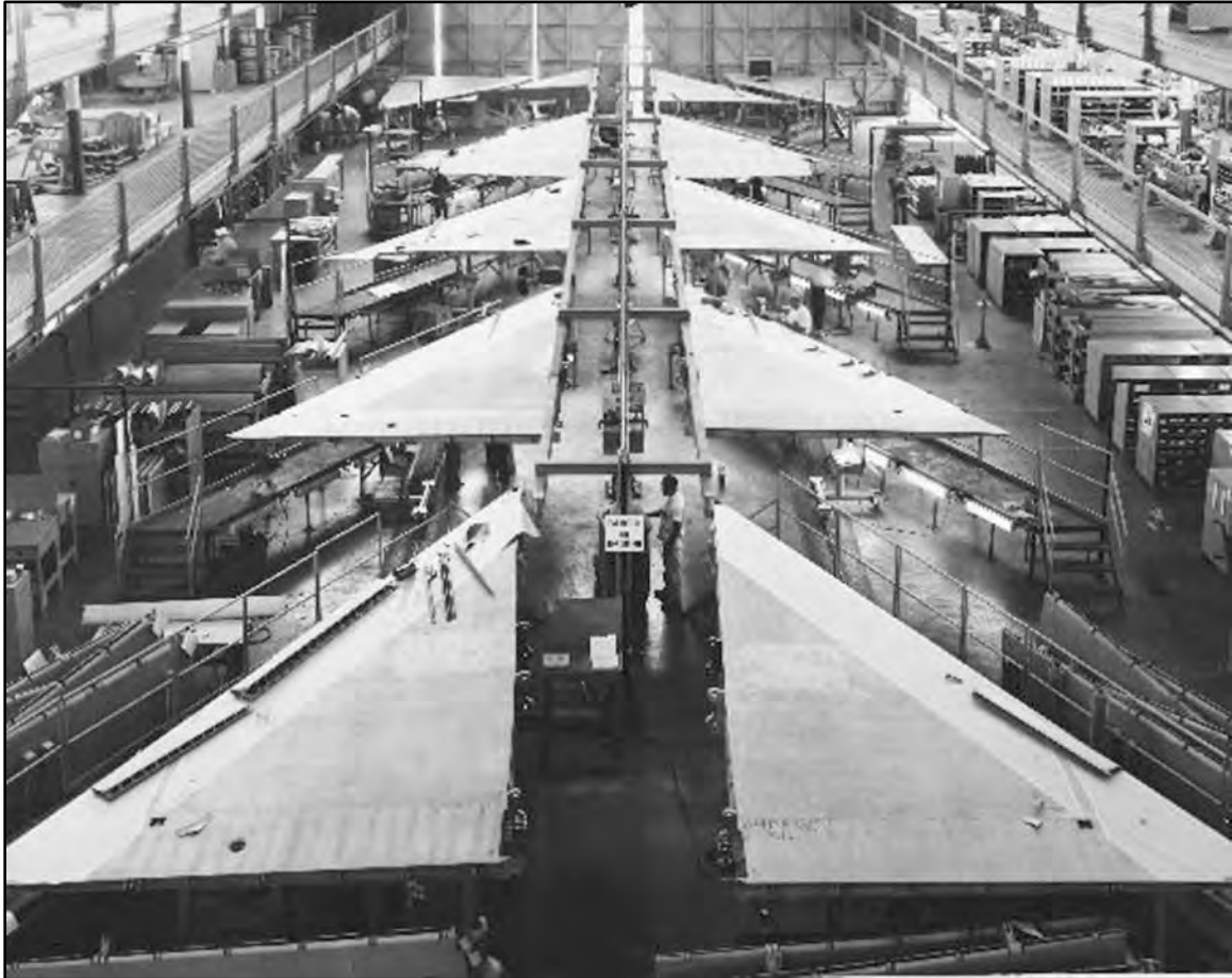
Figure 4.2-10 F-102 Assembly Line Showing Delta Wings Courtesy of San Diego Air and Space Museum.
