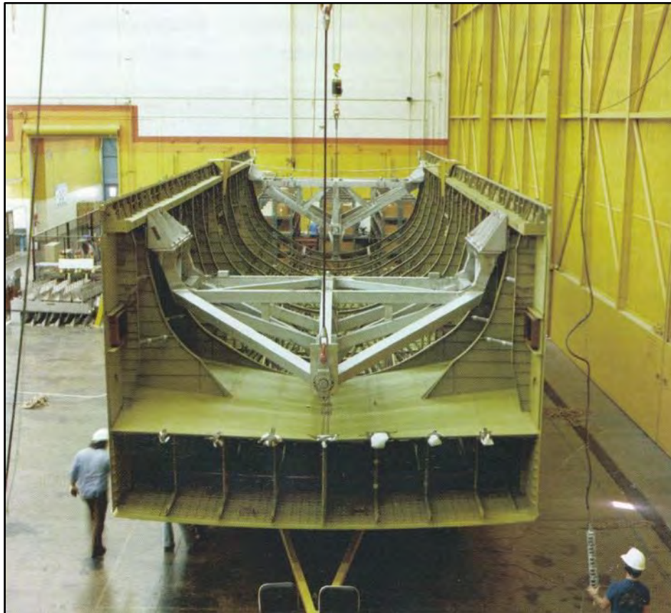
Figure 4.2-52 Mid-fuselage Mid-section Courtesy of David Baker, NASA Space Shuttle: Owners' Workshop Manual, p. 62.
