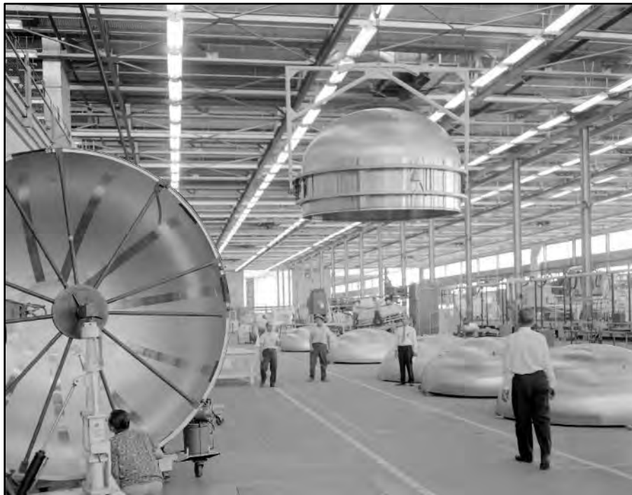
Figure 4.2-29 Moving Bulkhead by Crane, Building 3 (September 16, 1960) Courtesy of San Diego Air and Space Museum.
