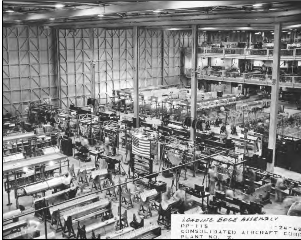
Figure 4.1-8 B-24 Leading Edge Assembly at Plant 2 (January 24, 1942) Courtesy of San Diego Air and Space Museum.
